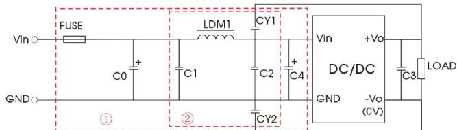
Notes: Part ① is used for EMC test and part ② for EMI filtering;
