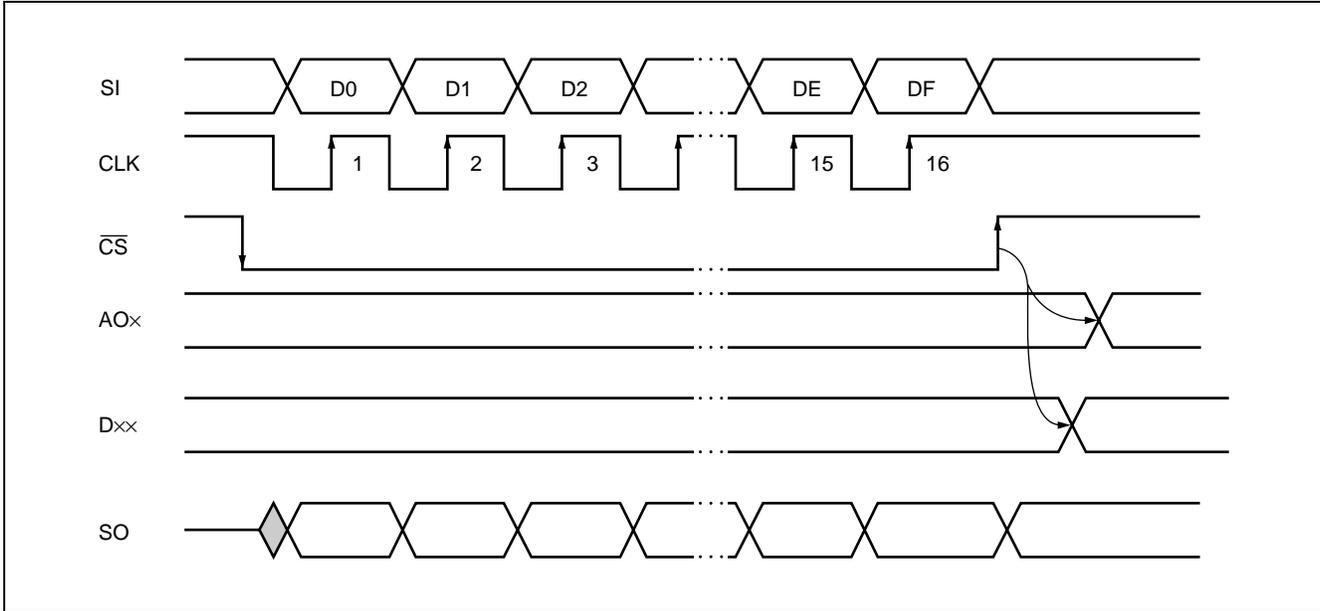
Data input is enabled at the falling edge of the  $\overline{CS}$  signal. 16-bit data is input, and the shift register command is executed at the rising edge of  $\overline{CS}$ .
