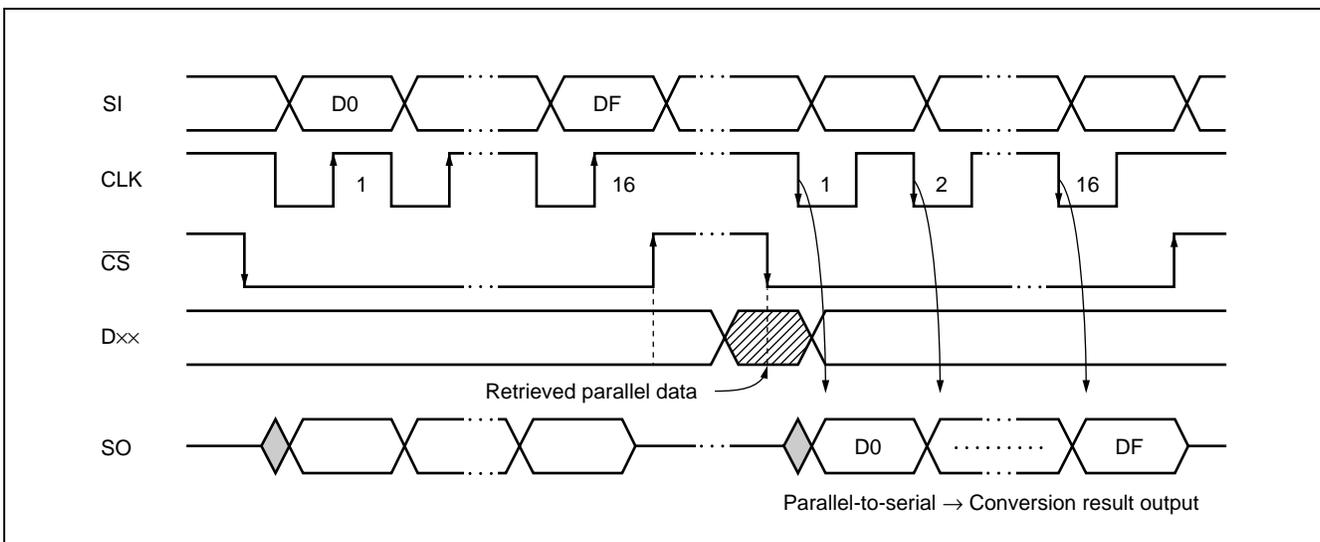
Data input is enabled at the falling edge of the  $\overline{CS}$  signal. 16-bit data (parallel → serial conversion commands) is input and commands accepted at the rising edge of  $\overline{CS}$ . At the falling edge of  $\overline{CS}$ , data from the parallel input is loaded into bits D4 to DF of the shift register, and output from the SO pin timed to the falling edge of the CLK signal.
