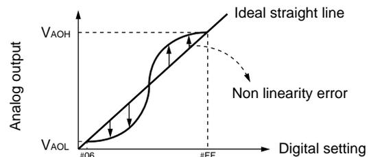
Note: The value of  $V_{AOH}$  and  $V_{DD}$ , and the value of  $V_{AOL}$  and GND are not necessarily equivalent.
